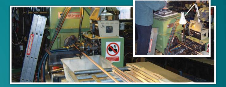
The HORMESA - Conticast® RF range of continuous casting machines are used for the manufacture of copper alloy, brass, bronze and zinc bars, tubes, sections and strip.
