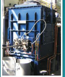
The HORMESA- Conticast® RV range of vertical continuous casting machines are used for the manufacture of oxygen free, high conductivity copper rod which is used to produce copper wire (C10200, ASTM B1, B2,
