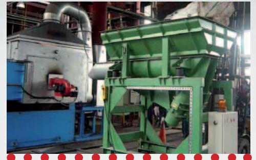
**Cargador vibrante** **Automatic vibrating charger**
